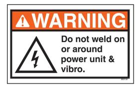
Do *NOT* weld on or around the power unit unless authorized in writing by APE. Doing so will void all warranties and may cause damage to the power unit or vibro.
